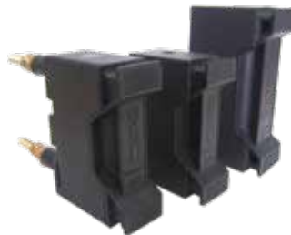
BBB Back stud connected (back-back) Mounting on board with two cables on the back (connection via lug. see table)
