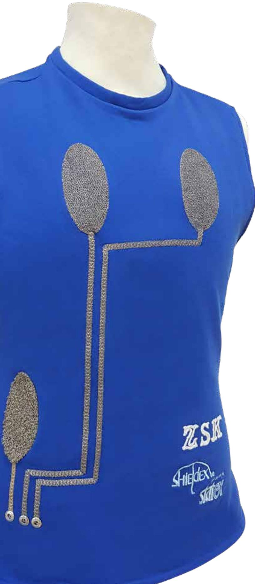
The K-Head creates moss embroidery. This single thread system creates loops at the surface of the carrier material. Voluminous surfaces will be generated by the compact placement of the stitches.
