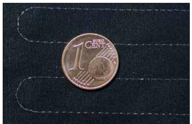
Fig.: Copper wire (70  $\mu\text{m}$ ) embroidered as bobbin thread
