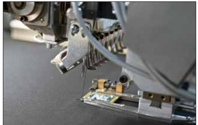
Fig.: Automatically placed Bosch PCB by ZSK PCB Placement Device
