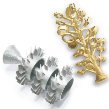
Casting trees in steel and in gold
