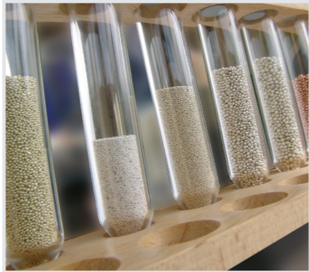
Micro granules in different alloys with a grain size of between 0.1 and 1 mm.
