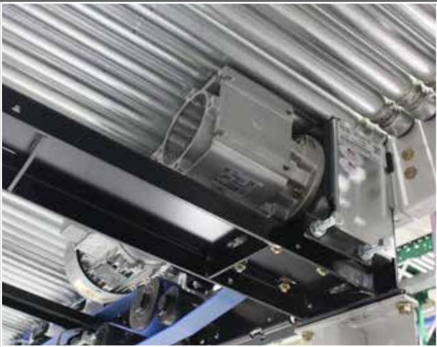
Low profile drive is designed for compact mounting (underside view)
