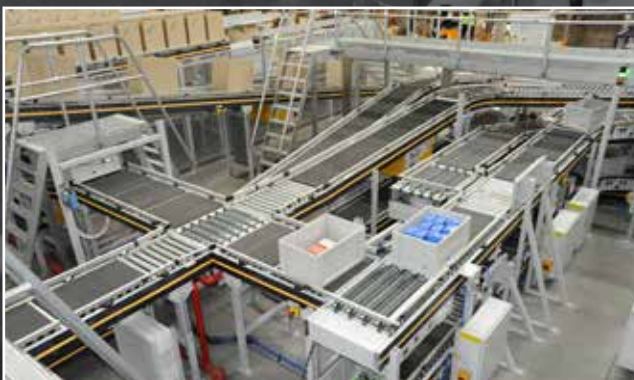
Segmented belt on roller accommodates apparel in poly bag
