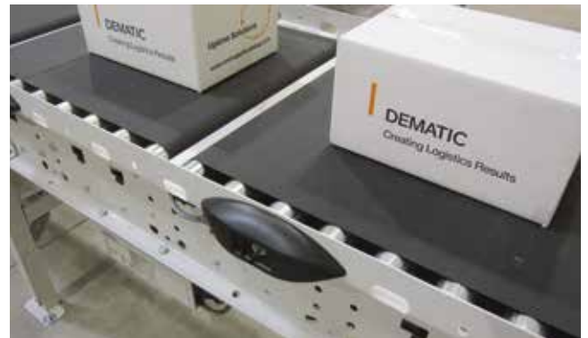
Housing protects electronic sensor
