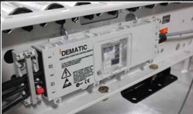
Embedded Conveyor Controller (ECC) controls the operation of motorised roller conveyordriven rollers
