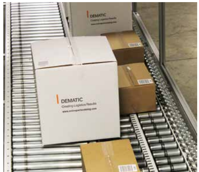
The singulator improves downstream merge and sorter performance
