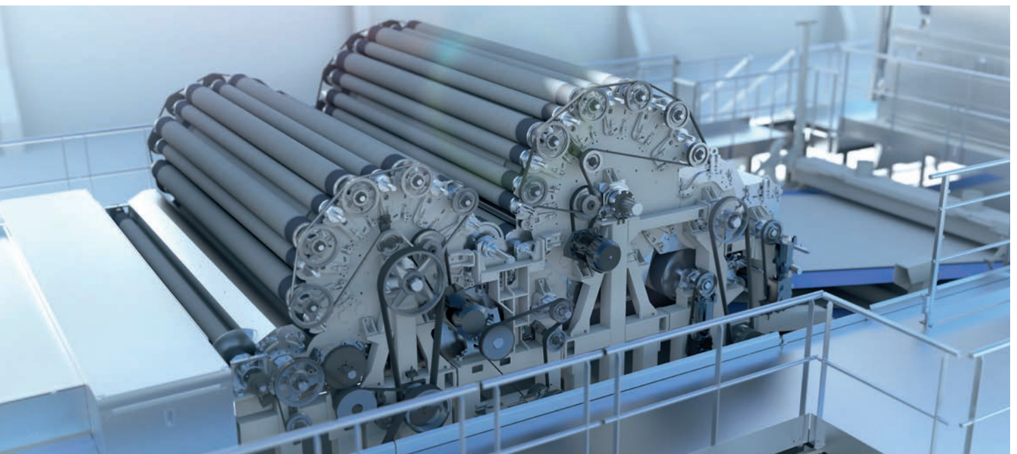
eXcelle TT card for high-speed spunlace lines
