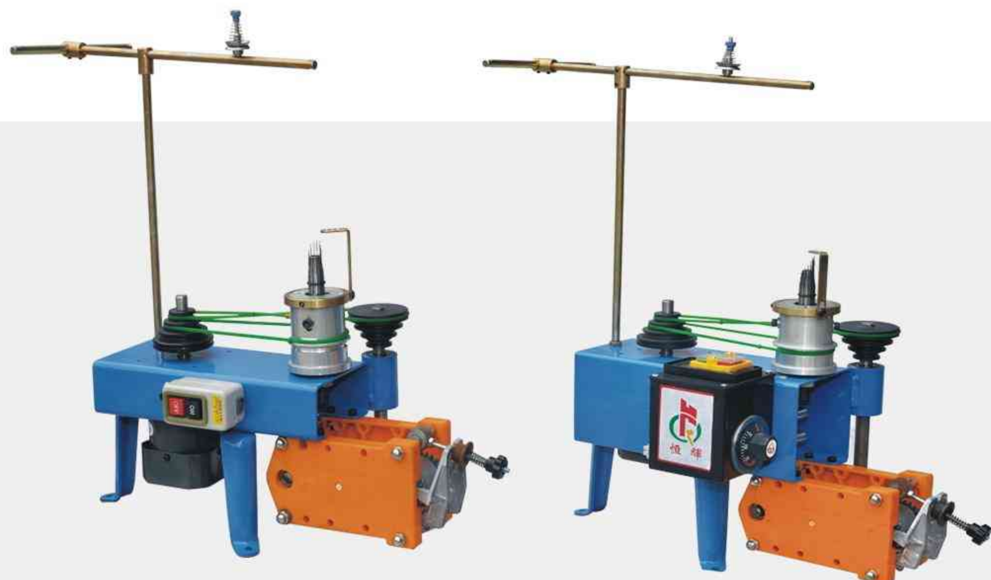
钩针机 Cord knitting machine (needle machine)
