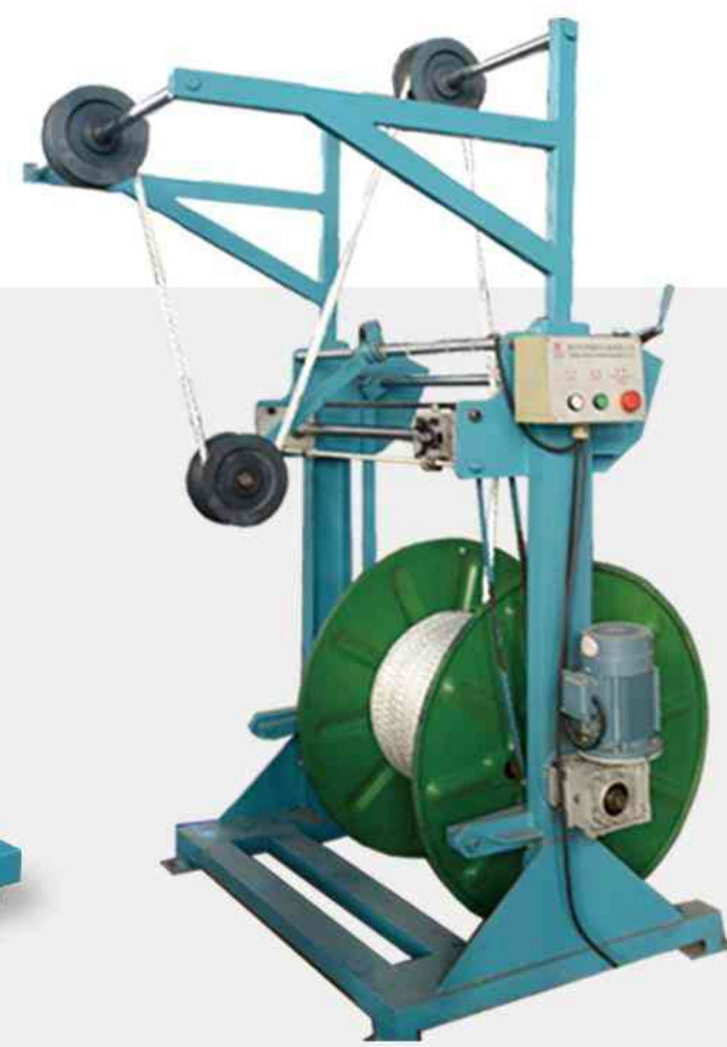
恒张力收线架 Constant tension take up device
