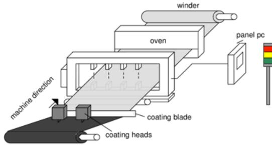
Fig. 6.b: An application case of M-Ray-based basis-weight measuring in a coating line.
