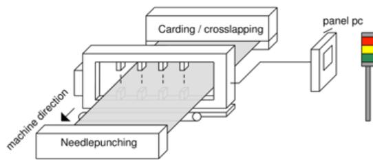
Fig. 6.c: An application case of M-Ray-based basis-weight measuring near the formation stage but before bonding. Thanks to the high stand-off distance of the technology, the gauge can also be positioned in the line where the web is still uncompressed, e.g. in between carding stages or cross-lapping stages.
