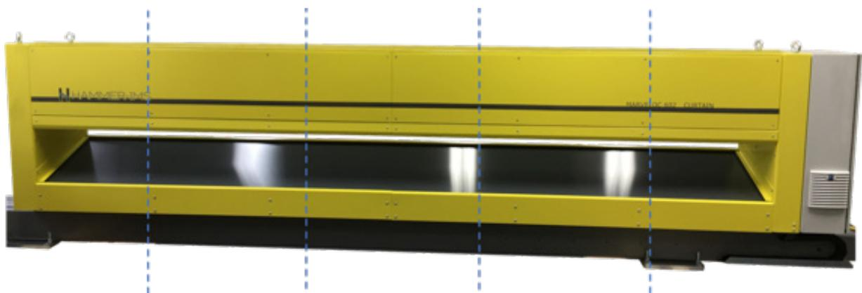
Fig.4: Industrial version of the Marveloc 602-CURTAIN-O basis-weight gauge. The 'CURTAIN' contains four measuring heads, as indicated by the blue dashed lines. This CURTAIN is more than 4.5 meters wide.
