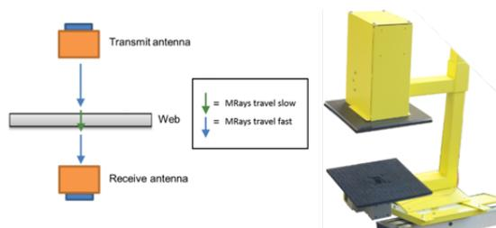
Fig. 1: Left: The concept of an M-Ray-based grammage gauge is similar to the one of a radar system. One antenna transmits a wireless wave, another receives it. The measured delay relates to the weight of the material. Right: an M-Ray-equipped C-frame for basis-weight measuring containing a single transmit-receive pair.
