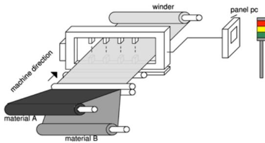
Fig. 6.a: An application case of M-Ray-based basis-weight measuring on a laminated product.
