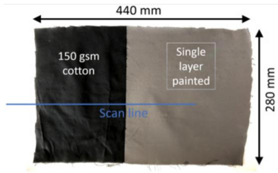
Fig. 8: Picture of the coated cotton sample which is used in the measurement results of Fig. 9. The blue line denotes the path the scanner has taken.
