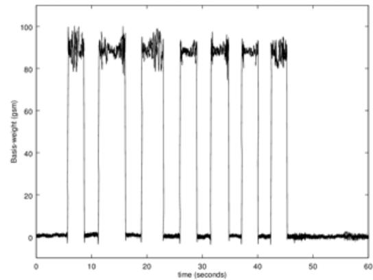
Fig.3: Graph showing the effect of repeatedly adding and removing a piece of copy paper in the measurement gap while continuously measuring a thick and heavy stack of various-colored synthetic nonwovens (thickness: 47 mm, basis-weight: 9.6 kg/m<sup>2</sup>). Note that the sensor is zeroed before introducing the piece of paper.
