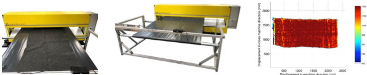
Fig.5: Experiments with a four-headed M-Ray system and belt drive, enables a full 2D view of a sample material [5]. Top: setup. Bottom: scan results.
