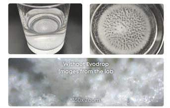
Aggressive limescale crystals form in the water and can easily deposit on surfaces.
