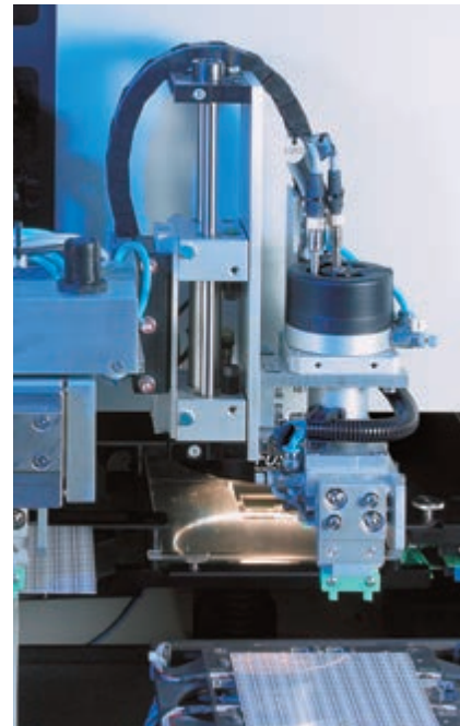
Laser trimming of platinum-chip temperature sensors
