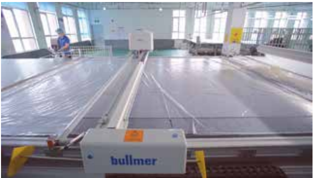
BULLMER AUTOMATIC CUTTING BED IMPORTED FROM GERMANY (3.2M WIDTH)
