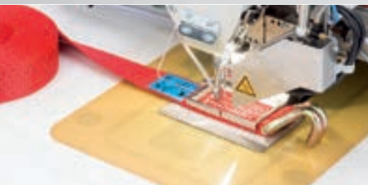
CNC-controlled sewing unit with template system for the production of lashing straps – sewing area of max. 200 x 100 mm
