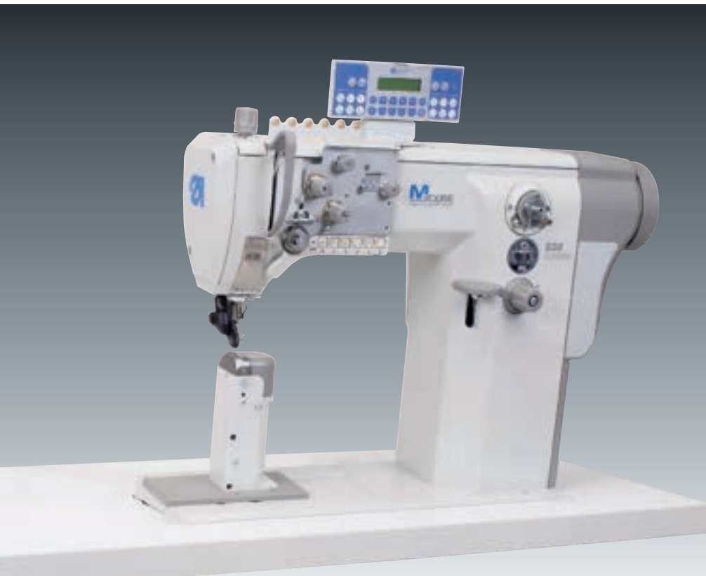
Single needle post bed machine with bottom feed for medium heavy materials
