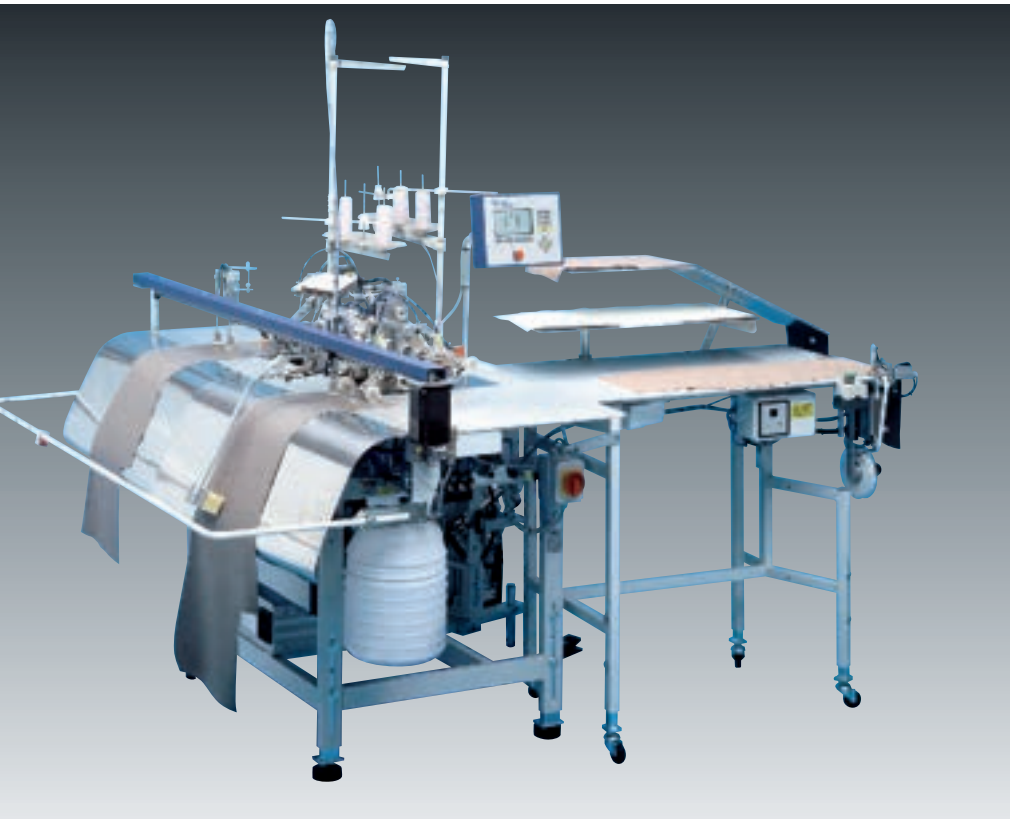
Twin head overlock unit – fully automatic serging of trousers, also in stretch material
