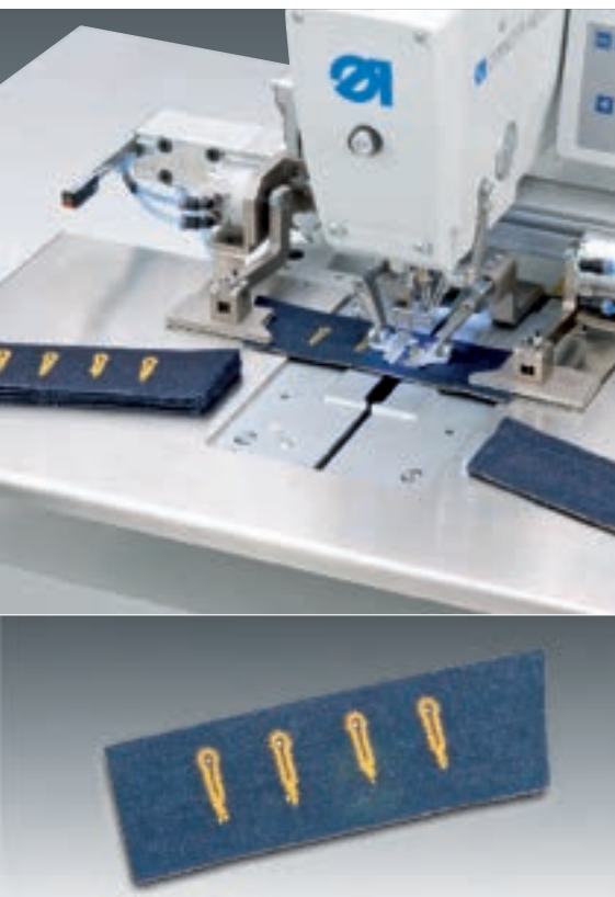
Eyelet buttonhole indexer for sleeve vents or small parts as e.g. jeans fly pieces
