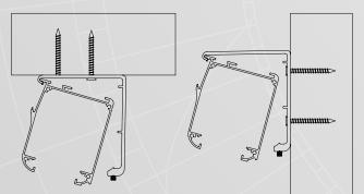
Wall and ceiling fixing is possible
